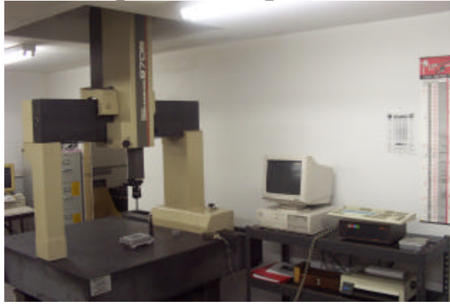
Mitutoyo B706 24" X 28" CMM Brown and Sharpe Micro Hite – with printouts Electronic Comparator – with printouts
